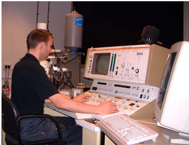
Scanning Electron Microscope being used to examine Solmax surface.
